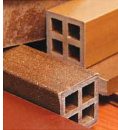
Eco-friendly furniture made from a wood polymer bio-composite of polypropylene and rice husks.
