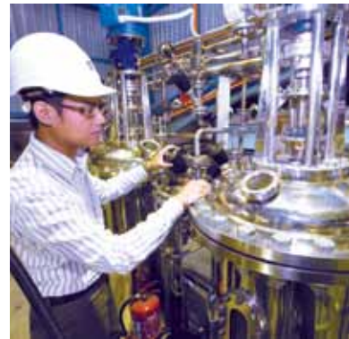
SIRIM's bioplastic plant turns oil palm waste into high-quality Polyhydroxyalkanoate (PHA) plastic.
