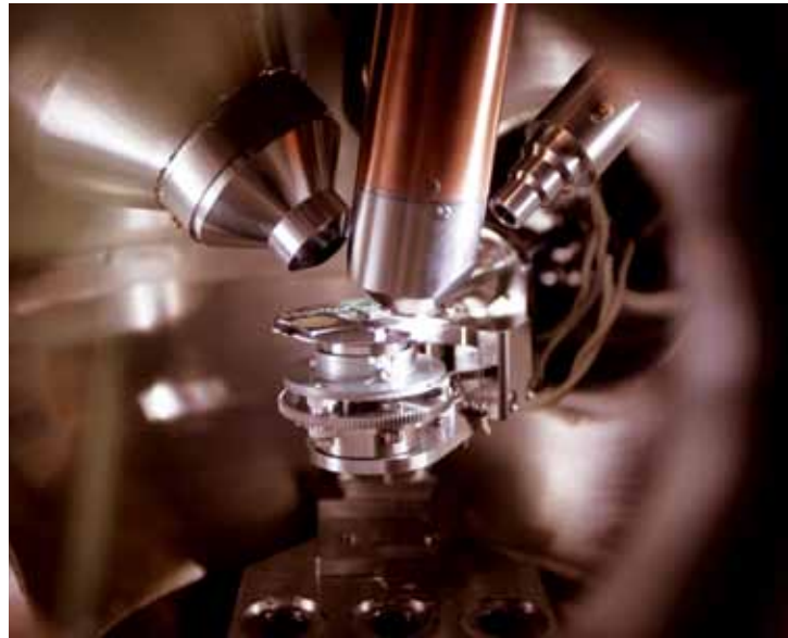
Researchers at SIRIM use an x-ray photoelectron spectrometer (XPS) to analyse the surface chemistry of biomaterials used in the company's medical products.
