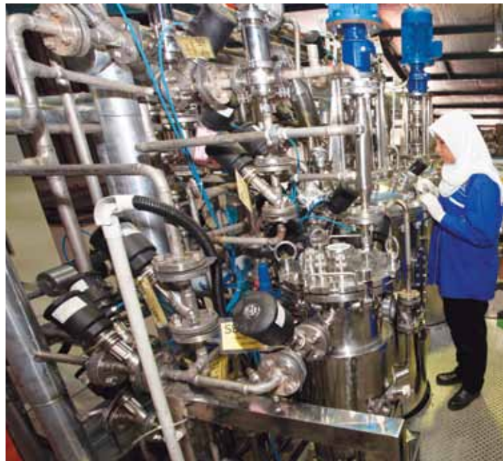
Pilot plants simulate the operating conditions of a full commercial plant.
