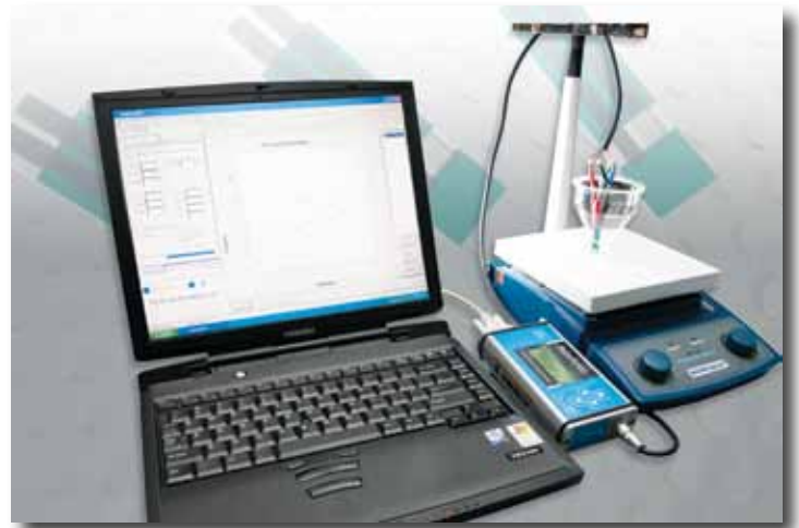
Bronze medal winner: Ammonium Monitoring System for Sustainable Aquaculture Industries , an optical sensor that monitors ammonia levels in aquaculture ponds. The sensor will be used in SIRIM's Green Aquaculture System.
