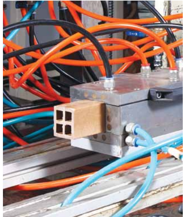
ONE LEG AT A TIME: SIRIM's bio-composite material is heated and then pushed through a die to produce long profiles that are then cut into various lengths depending on the requirements of the furniture.
