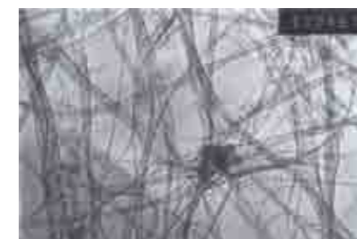
MIDDLE: A TEM image of Single-Walled Nanotubes; 90wt% purity; 1-2 nm outer diameter; 5-30 µm length
